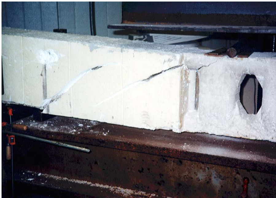
Figure 7a Typical Failure Mode for the Long-Span ICF Screen-Grid Lintel (6x12 specimen)
