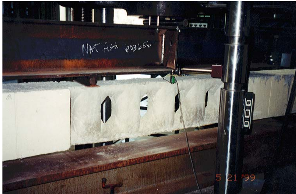
Figure 4 Steel I-Beam, Loading Points, and Deflectometer
